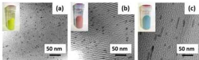
**Fig. 1** TEM micrograph of size and color controlled Ag/SBA-15 (a) yellow (b) red (c) blue
