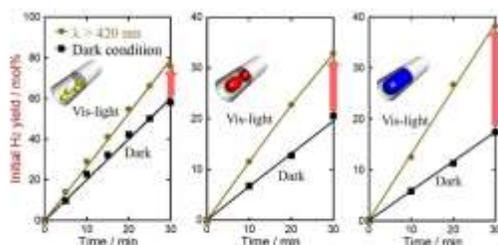
**Fig. 2** Time course of hydrogen production by Ag/SBA-15 in dark (●) and under light radiation (■)
